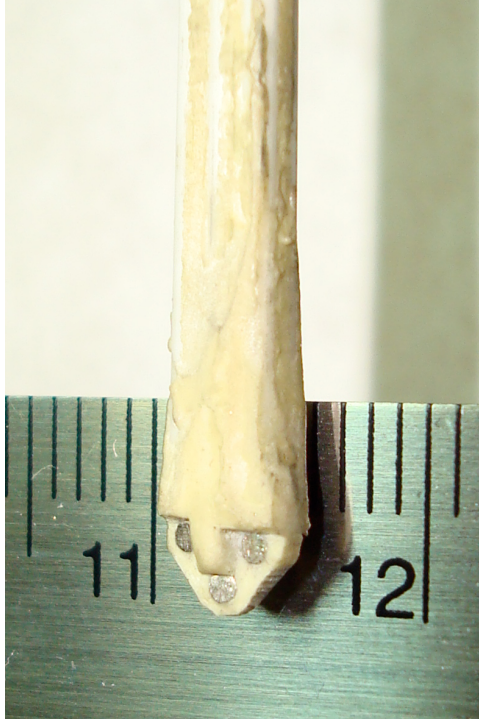
Figure 2.9: Head of a two-sided triple probe placed against a ruler (cm scale). Three disc tips are visible, with another set of three on the other side.
